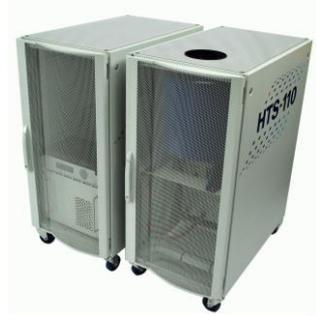
Fig. 1 200MHz mobile NMR system
